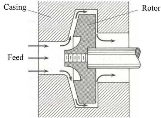
**Figure 5.9: Schematic drawing of colloid mill**
