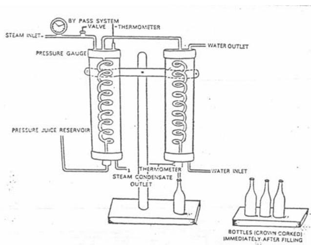
Figure 9.10: Schematic representation of a flash pasteurizer
