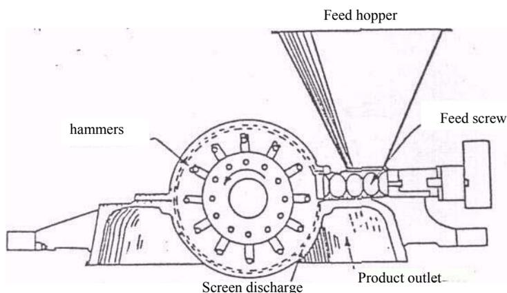
Figure 9.5: Sectional view of hammer mill
