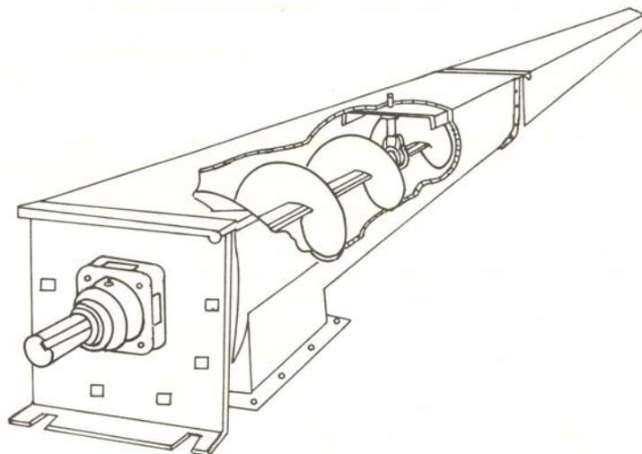
**Figure 7.3a: Screw conveyor**
