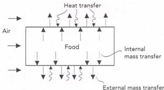
Figure 1.20: Principle of drying of food
