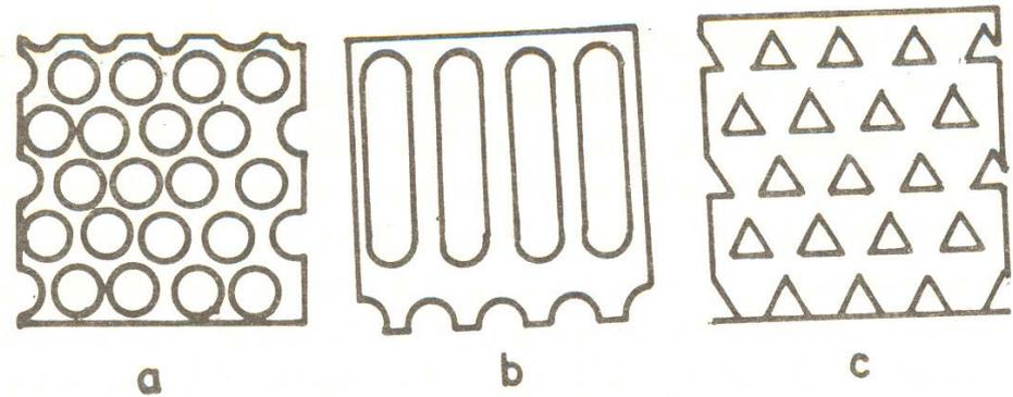
Figure 3.16: Perforated metal screens. a) Round holes, b) Oblong holes, c) Triangular holes
