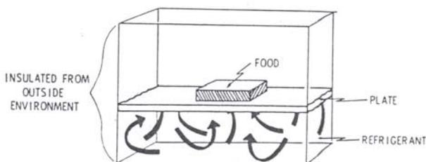
Figure 1.10: Schematic diagram of indirect contact freezing
