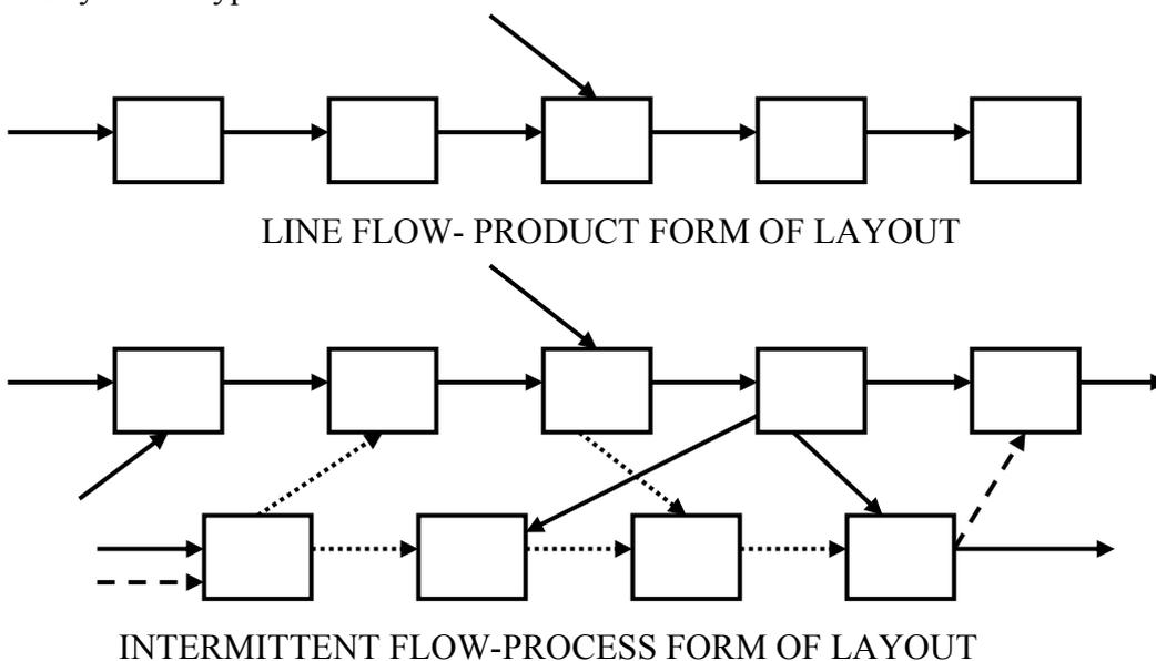
Figure 13.3: Product form and process form of layout
