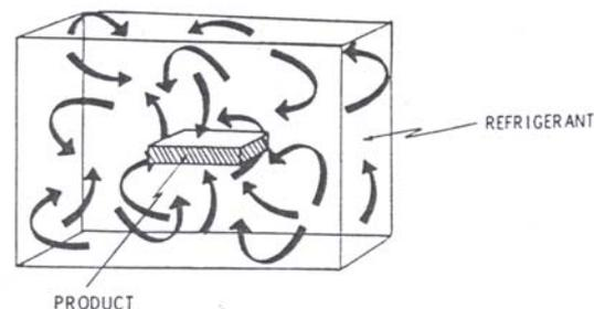
Figure 1.11: Schematic diagram of direct contact freezing
