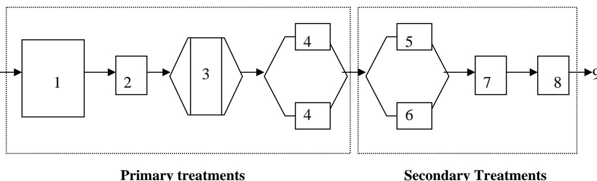
**Figure 15.1: Waste water treatments: 1) Screen, 2) Shredder, 3) Grit chamber, 4) Primary sedimentation tank, 5) Trickling filter, 6) Activated sludge tank, 7) Secondary sedimentation tank, 8) Chlorination tank, and 9) final effluent.**
