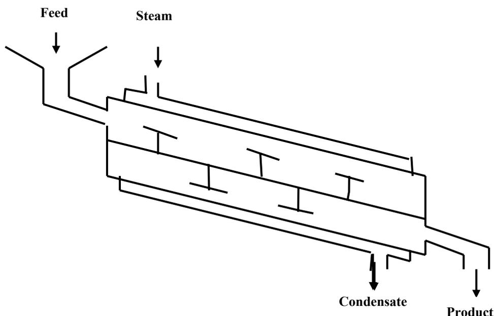
Figure 12.14: Rotary dryer
