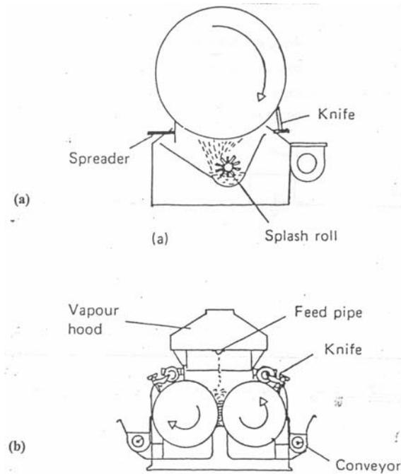
Figure 12.11: Drum driers: a) Single drum, b) Double drum
