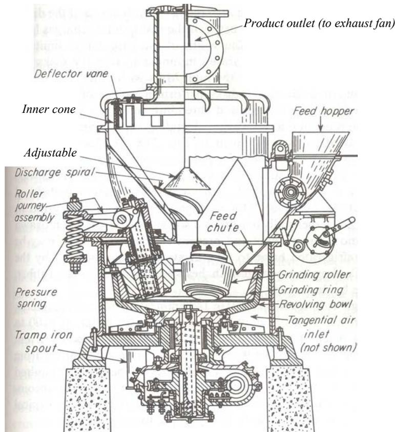
**Figure 5.6: Roller mill**
