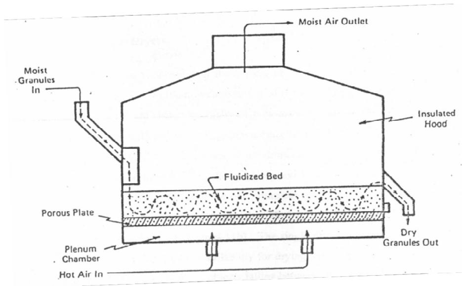
Figure 12.10: Schematic illustration of fluidized bed drier
