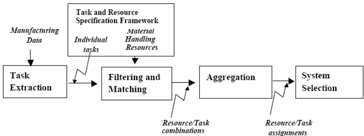
Figure 7.11: Major steps of procedure for selecting and specifying material handling equipment for manufacturing.
