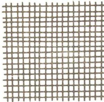
Figure 3.17: Wire mesh screen (square openings)
