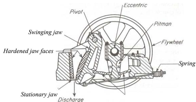
**Figure 5.1: Jaw crusher**
