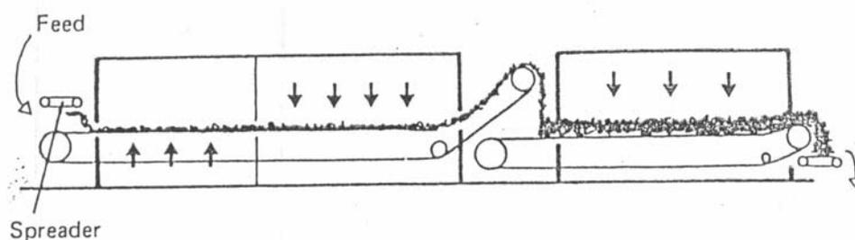
Figure 12.9: A typical two stage conveyor drier/belt drier
