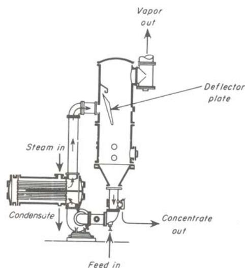
Figure 1.18: Forced circulation evaporator
