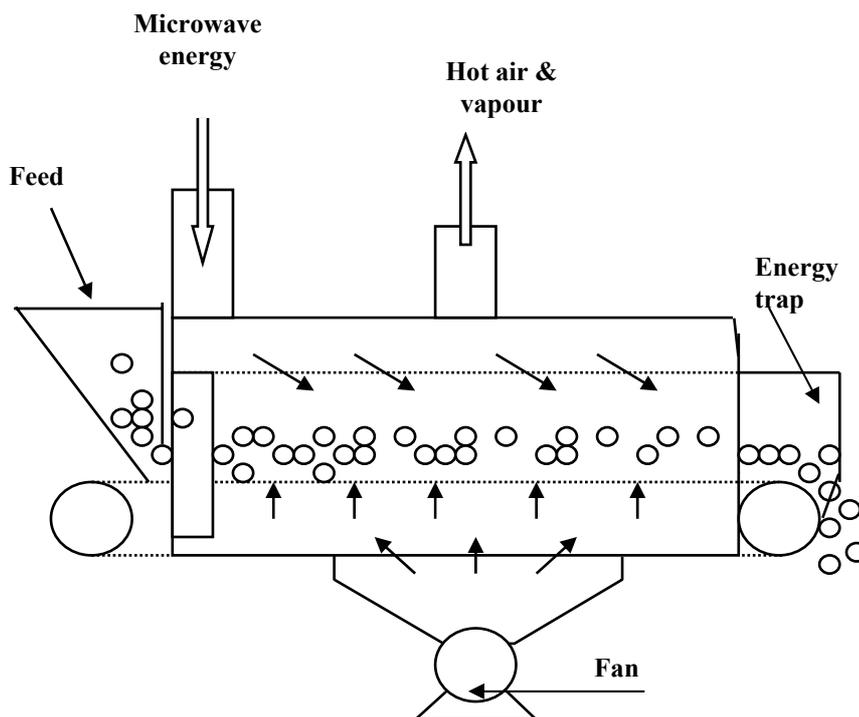
**Figure 12.13: Schematic of a continuous microwave drying equipment**
