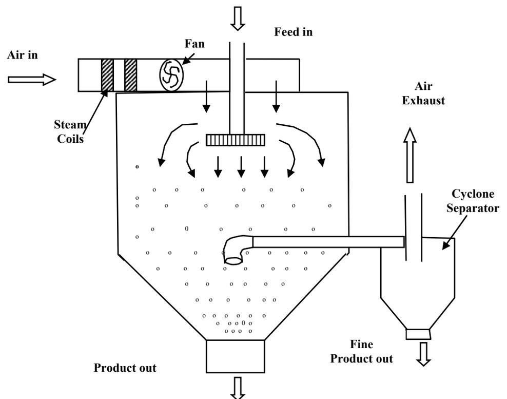
Figure 12.12: Typical schematic arrangement of a spray dryer
