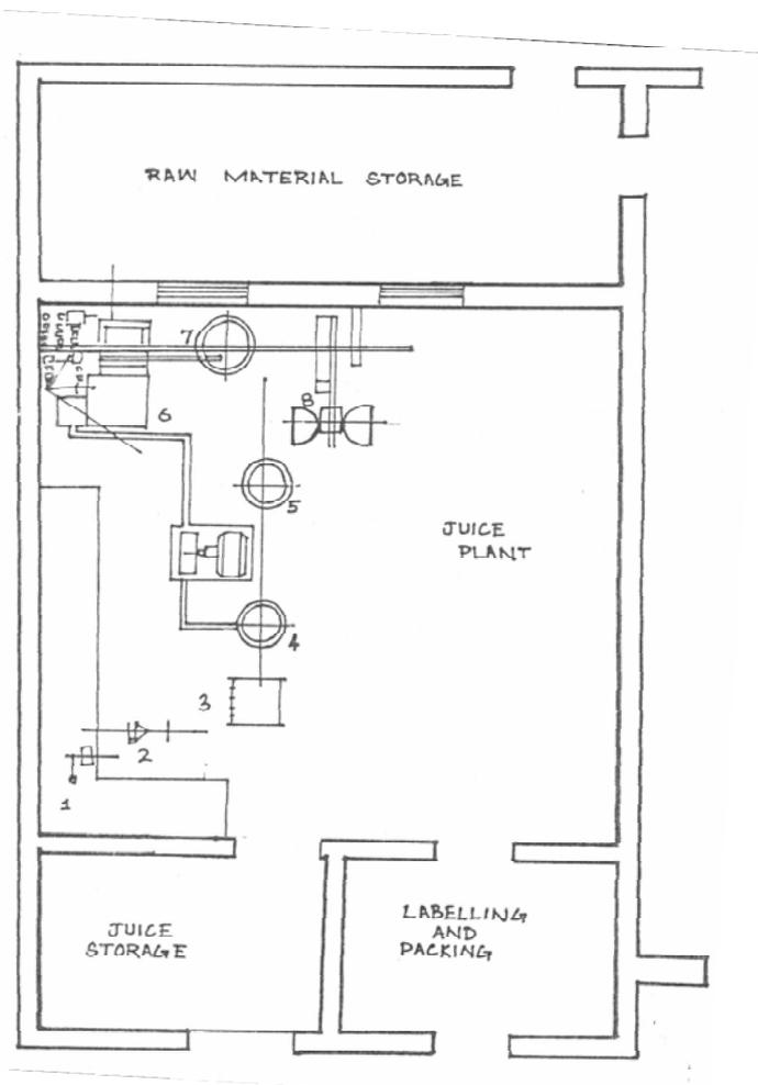
**Figure 13.5: Layout plan of a fruit juice plant: 1) Capsular, 2) Corker, 3) Filler, 4) Syrup agitator, 5) Syrup maker, 6) Pulping M/C, 7) Pump, and 8) Pulp extractor**
