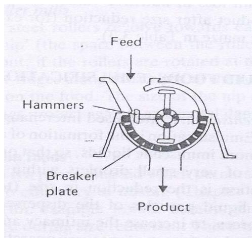
**Figure 6.5: Hammer mill**
