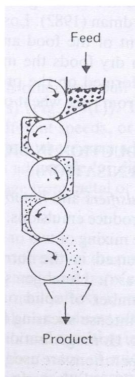
Figure 6.6: Roller mill
