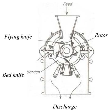
Figure 5.10: Rotary knife cutter
