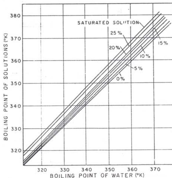
Figure 1.12: Duhring lines for sodium chloride – water system
