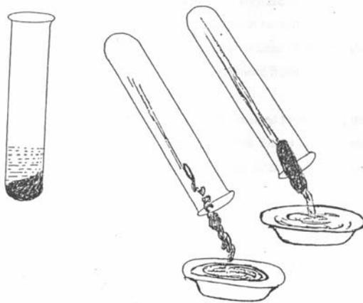
Figure 10.4: Pectin test for jelly extract. a) Low pectin extract; b) High pectin extract
