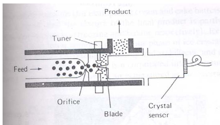
Figure 6.8: Ultrasonic homogenizer
