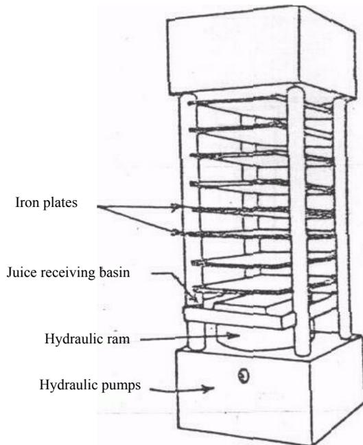
**Figure 9.8: Schematic diagram of a hydraulic juice press**
