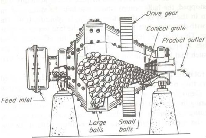
Figure 5.8: Conical ball mill
