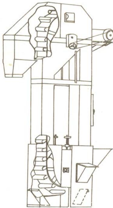
**Figure 7.8: Bucket elevator**
