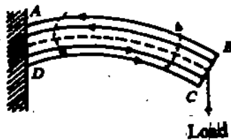
Fig. 6.5: When the beam is bent then in the upper half, the restoring forces opposing extensions in the filaments act inwards towards the fixed end. While, in the lower half, the restoring forces opposing contractions act outwards. The moments of these two set of forces about the neutral axis are directed in the anticlockwise (indicated by dotted arrows) direction and thus oppose the bending of the beam.
