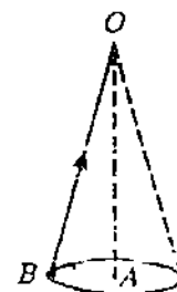
Fig. 9.9: B is the bob of a conical pendulum and OA, the axis of rotation.
