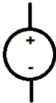
Fig 10.16 Constant Voltage Source symbol
