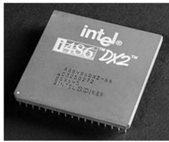
Figure 7: An Intel 80486DX2 CPU, as seen from above
