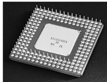
Figure 6: Bottom side of an Intel 80486DX2 1
